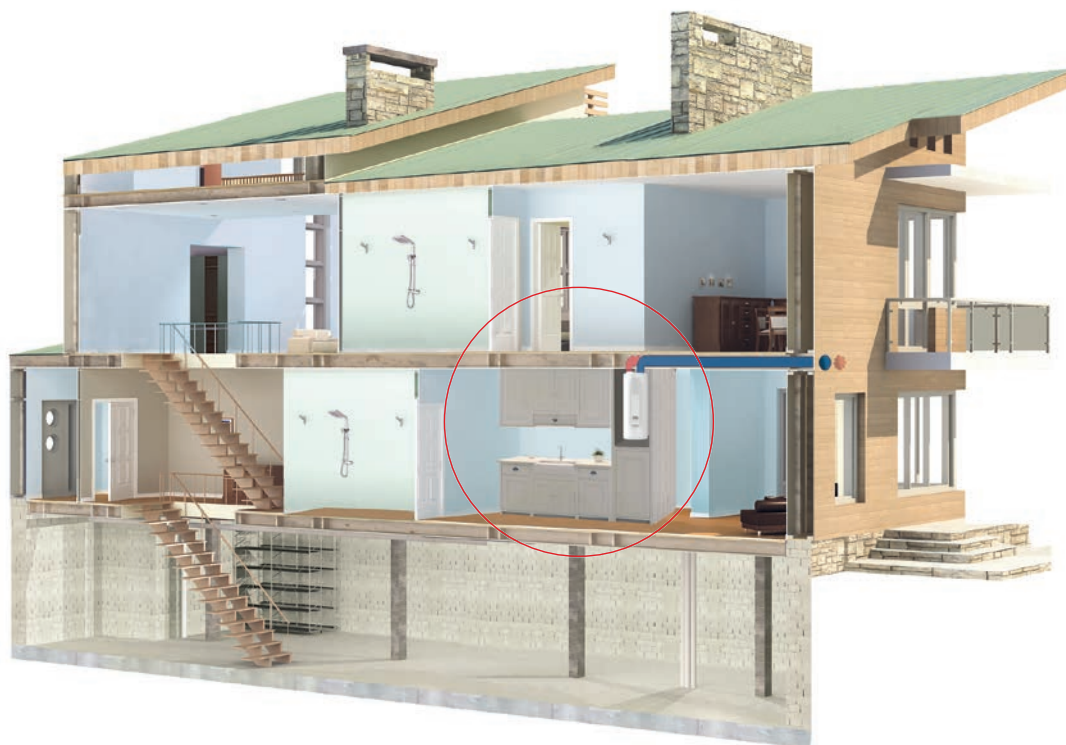
Installation with internal air intake: with air extraction outdoors.
