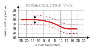
**2. MANUAL SETTING:** The inlet temperature can be set manually between 20 $^{\circ}$  C and 52 $^{\circ}$  C.
