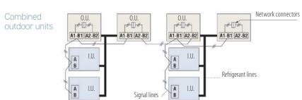
The maximum number of indoor units that can be connected to a signal line is 128, and it is possible to create groups of outdoor and/or indoor units connected to the same outdoor unit or to separate outdoor units, as long as they are connected to the same signal line. The signal line can also be connected by adopting the method described below (multiple connectors).
