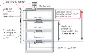
With difference of length between the farthest indoor unit and the nearest one from the first branch pipe < 40 m (MAX 85 m).
